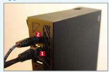
To get started, connect the storage device to your router using the supplied Ethernet cable, 11 then attach the power. 2 The device will configure itself. This can take up to 10 minutes, after which the blinking light on the front of the box stops flashing and the device is ready to use.
